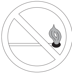
Fig. 6 - Do Not Light Burner with Match
